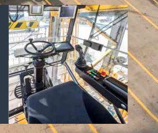
be handled simultaneously. All of our shuttle carriers are easy to operate and have servicing intervals of up to 1000 hours, keeping your machine's downtime to a minimum. Plus, all servicing points are easily accessible from the top of the frame.
